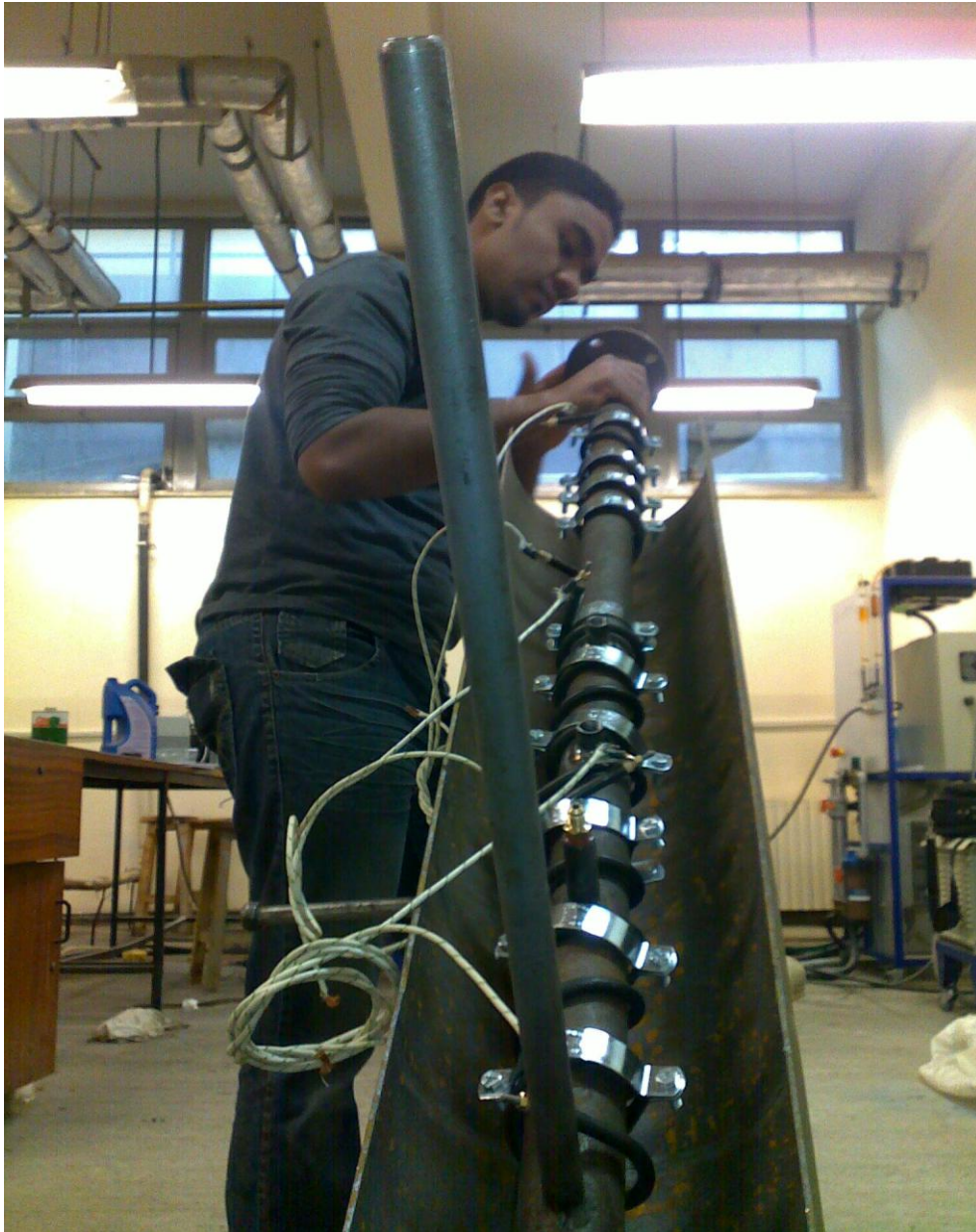
Figure 4.6: Electric heater coil installation around shock tube
